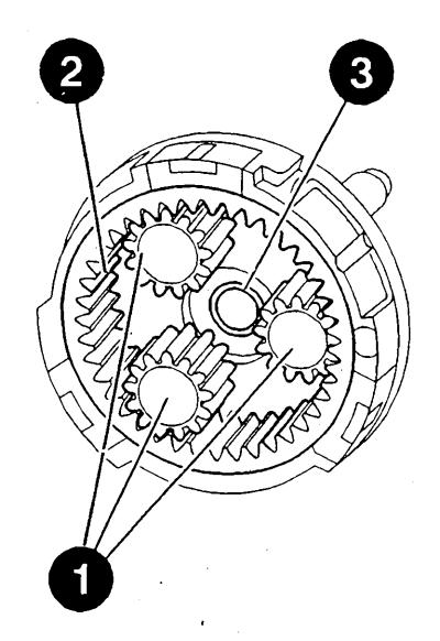
Checking planetary gear train
